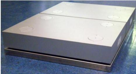
PIATTAFORMA A SECCO STRUMENTATA CON PEDANE DINAMOMETRICHE PER LA MISURA DELLE FORZE
